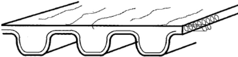
3. A crack reaches from the base of a cog of a timing belt to the rubber layer.
